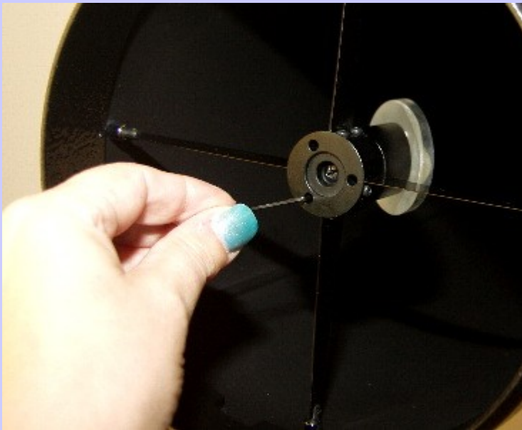
Adjusting the secondary mirrors 'tilt'.
