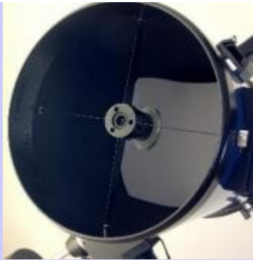
White card inserted into telescope tube to block reflections in the secondary.
