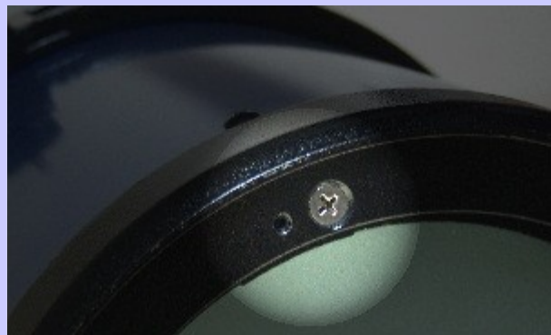
Collimation screws. Lock screw to left, adjuster to right (differs between telescope manufacturers).
